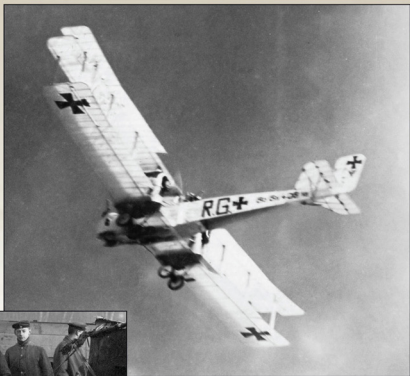
^ This photo of Gotha G.IV 406/16 in flight allows us to see the highly translucent nature of the bleached linen wing and tailplane covering (including the lower wing center section B1 ). (Thomas Genth)
