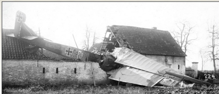
This unfortunate LVG built Gotha G.IV (LVG) 991/16 'MoRoTAS' struck a Belgian farmhouse on the night of 10-11 November 1917. Initial production G.IVs from LVG like this one retained most of the Gotha built aircraft features, some exceptions being the propeller guards, alternative control cable guide locations on the fuselage and additional tailplane struts. The letters on the side of the fuselage stand for Lt. Mons (or Mongis), Lt. Roland and Herman Tasche. We have illustrated these letters as black, white and red rather than as conventionally illustrated red, white and yellow because we feel the tones match better and because there would be no need to have a white outline around yellow letters on a dark painted fuselage like this, but it would make perfect sense around a darker colour such as red. Tasche evidently survived this incident with the farmhouse because on the evening of 9 May 1918 he appears to have been the sole survivor of a Gotha G.V(?) shot down over England by a 141 Sqn Bristol Fighter crewed by Lieutenants Turner and Barwise. A photo showing the other side of this incident is shown on page 20 of Gotha!
