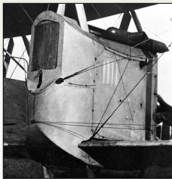
Another view of Gotha G.IV 603/16 showing further interesting details like the double control cables for the ailerons and the non slip tread walk area on wing. Note the wire threaded through the nacelle turn buttons to prevent them working loose in flight.
