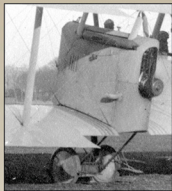
Engine nacelle details visible in this close up of Gotha G.IV 406/16 are the air intake (D11) and the single set of cooling louvers common to Gotha built G.IVs. (Thomas Gent)
